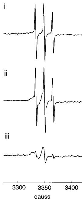
FIGURE 8: ESR spectra obtained for the nitroxide-labeled fatty acids, in which the spin probe has been attached at the carbon 5 and 12 positions at the acyl chain and incorporated in DMPC/PDA vesicles (total lipid concentration of 1 mM): (A) 5-DS and (B) 12-DS. The peptide:lipid ratios were (i) 0, (ii) 0.05, (iii) 0.1.
